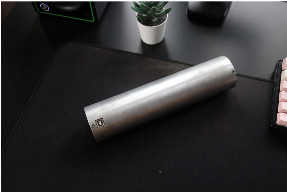
Figure 2.1: NaI(Tl) crystal-based sensor
